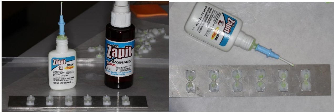
Figure 8. Beams were glued with a cyanoacrylate adhesive (Zapit Dental Ventures of America, Corona, CA) to Microtensile Geradeli Jig 2
